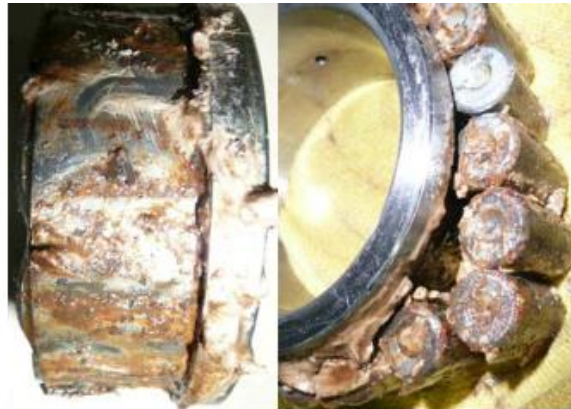
Corrosion. Contaminated lubricant.
