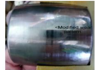
Abrasive wear on rollers raceway.
