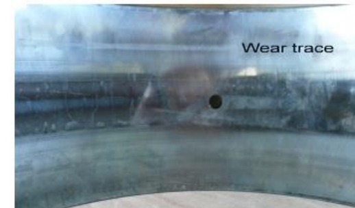
Abrasive wear on outer ring raceway ( SRB).
