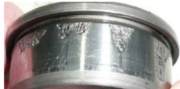
Flaking due to vibration (equally spaced at roller pitch).
