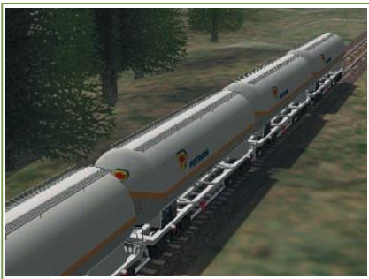
Freight wagons with Y25 bogies
